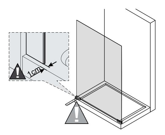
▶ Install the seal rubber on the down side of the glass, so the rubber will be between the glass and the tray.
