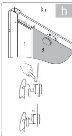
► Hang the doors on the upper guide and lock them by pressing the springs on the lower rollers to apply appropriate and in the lower guide.
