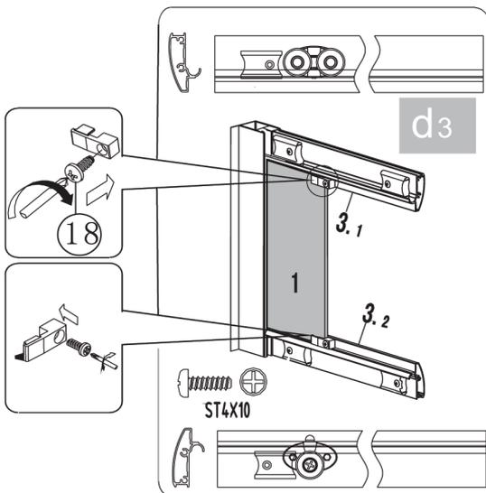
► Secure by screwing the special clips on the horizontal guide on the one hand.
