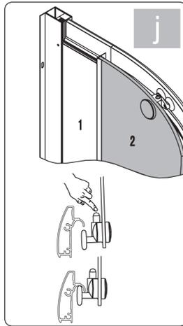
► Hang the doors on the upper guide and lock them by pressing the springs on the lower rollers to apply appropriately and in the lower guide.
