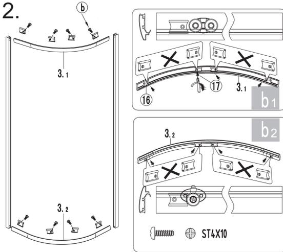
► Screw the horizontal guides to the vertical profile bearing the special recess for stable crystal in order to set up the metal frame.
