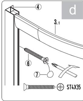
► Place in the frame the stable glass within the vertical profiles that you have been already screwed to the wall.
